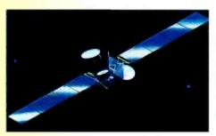
Satellites: Positioned 22,300 miles above Earth, the company's three satellites beam programming and information directly to subscribers' small satellite dishes. The three birds are approximately five times stronger than traditional satellites and transmit up to eight times as many video signals.
